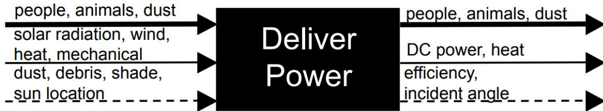
Figure 2: Black Box Model of NMSU solar panel system
